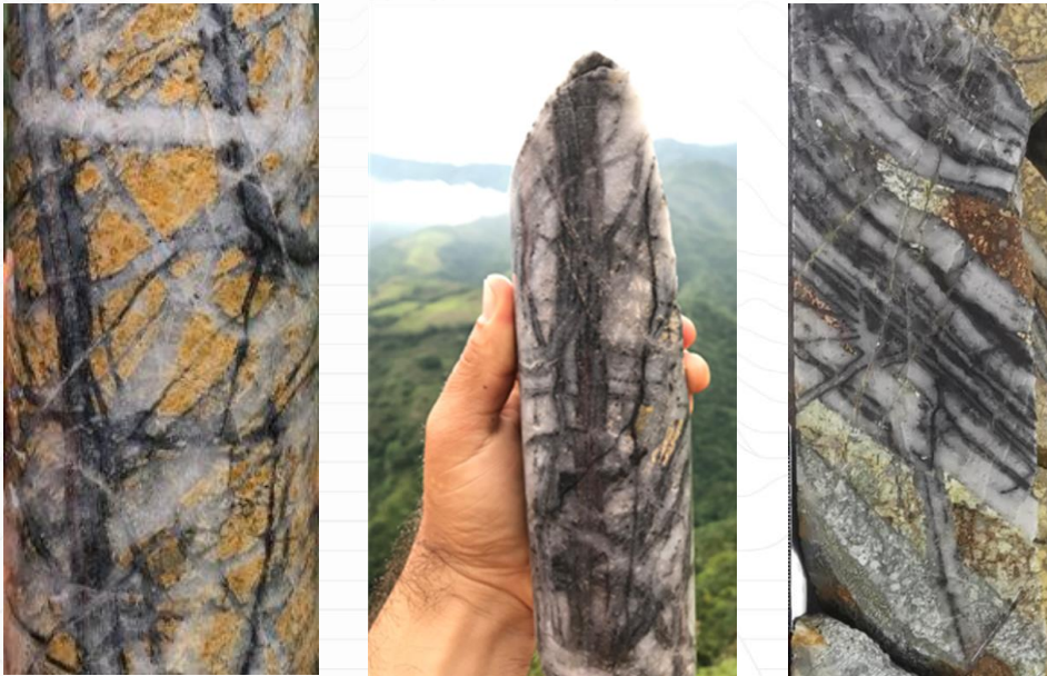
High density banded porphyry quartz veins with phyllic, intermediate argillic overprint
