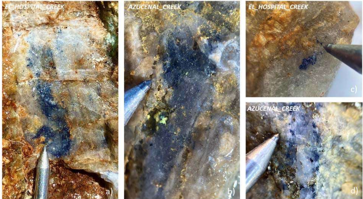
Figure 7.16 Veinlets of quartz-pyrite-chalcopyrite-molybdenite.
