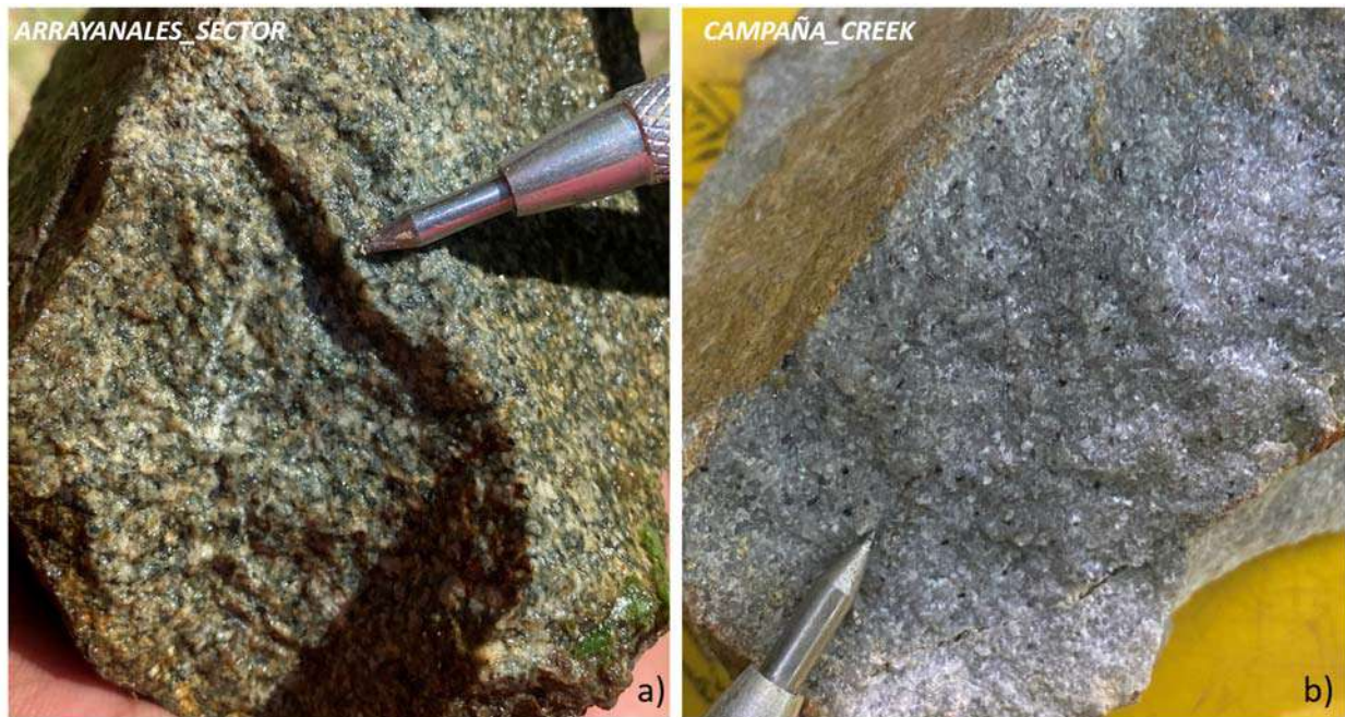
Figure 7.4 a) Medium grained diorite; b) Fine to medium grained diorite.
