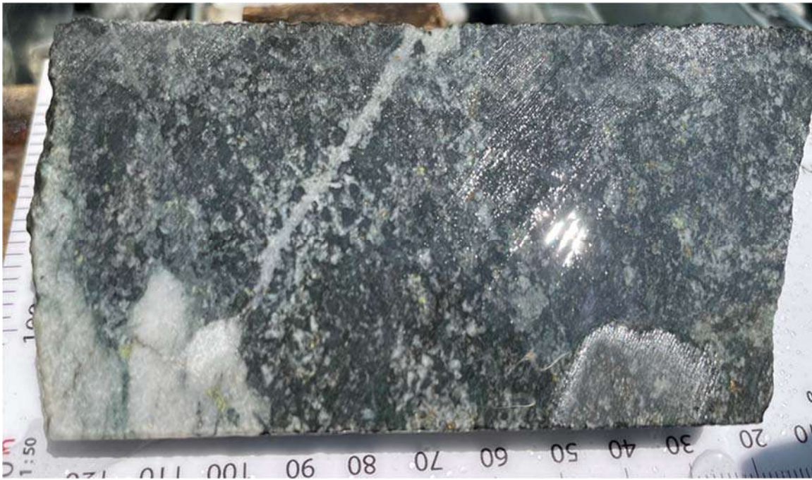
Figure 7.12 Strong biotite-magnetite alteration of diorite in SA-18-01 at 586.80 m.
