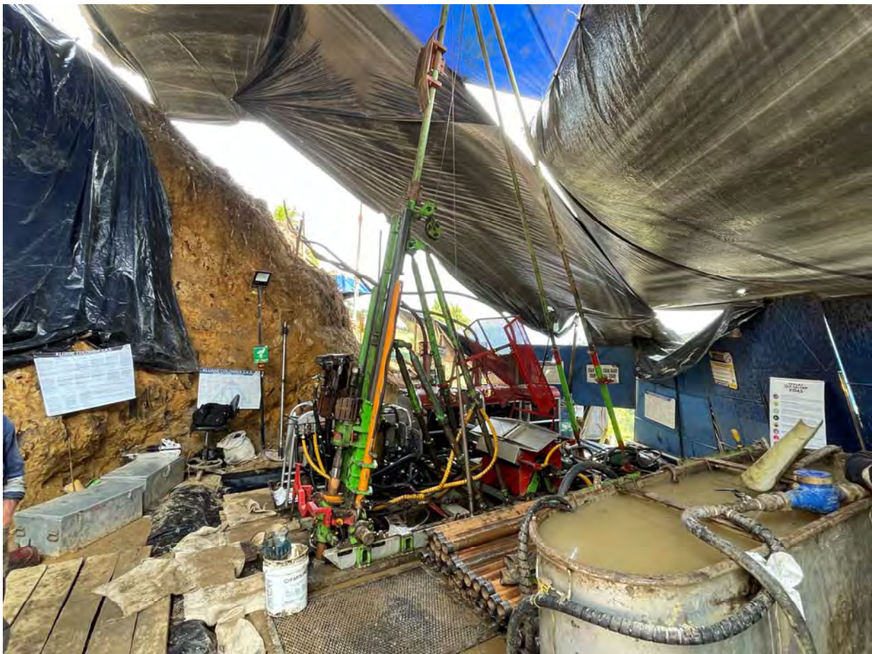
Figure 10.2. Portable Kluane KD-1000 hydraulic drill rig drilling hole APC-031 on Drill Pad 6 on 14 January 2023.
